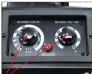
(14) Set welding parameters using the voltage and wire feed controls.
