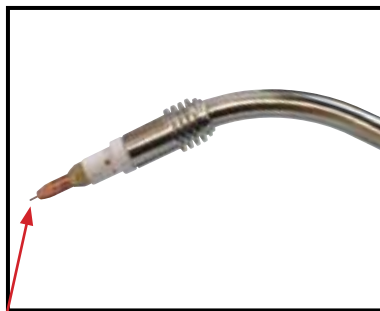
(17) Fit an Aluminium contact tip of the correct size to match the wire diameter being used
