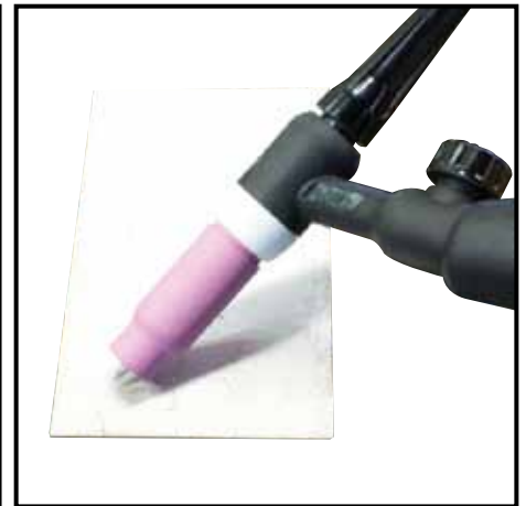
(7) Lay the outside edge of the Gas Cup on the work piece with the Tungsten Electrode 1- 2mm from the work piece.
