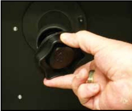
(1) Remove the spool retaining nut.
