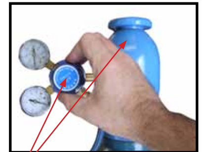
(13) Carefully open the valve of the gas cylinder, set the flow to 10-15 l/min
